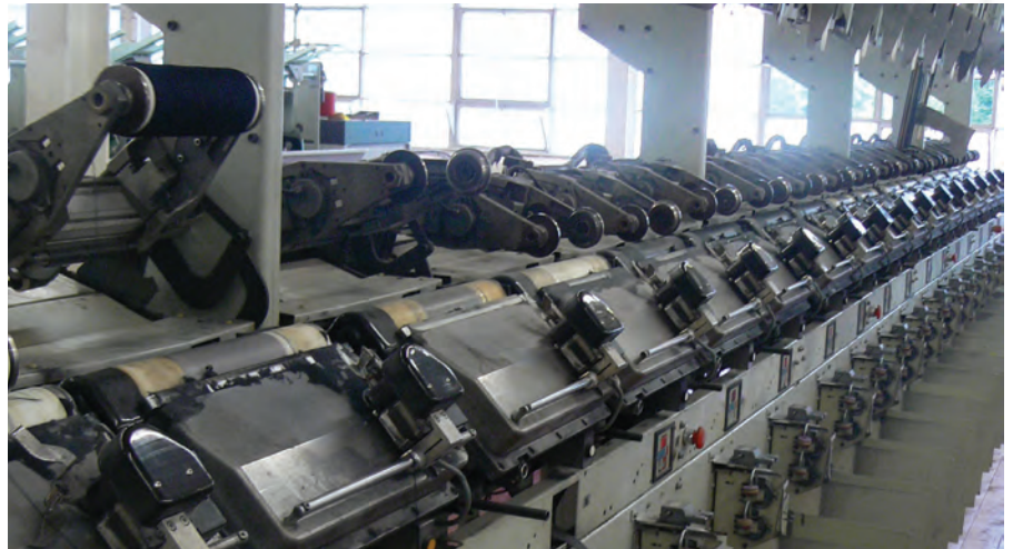
Measured length winding strips down the yarn from large to small cones according to the warp required.
