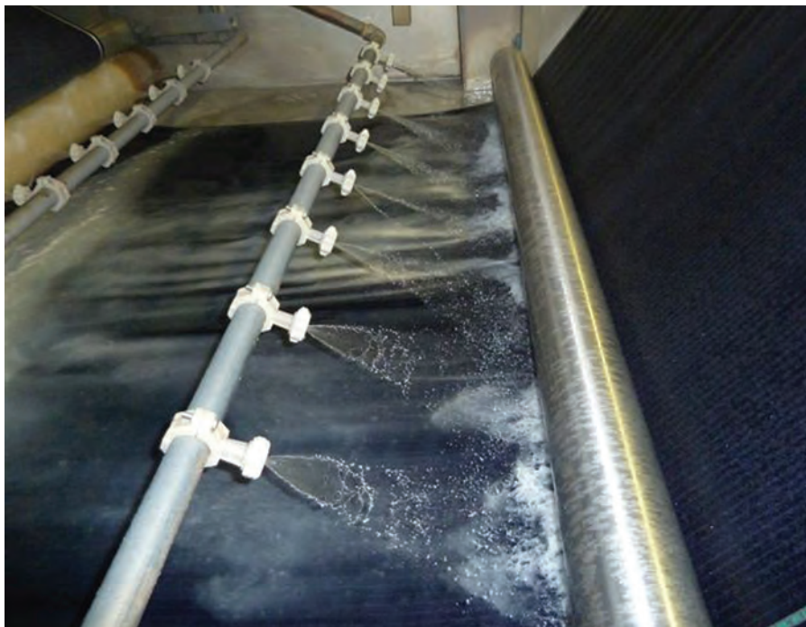
The jade is ground down into a powder and made into a suspension through the addition of water. The suspension is then sprayed onto the cloth, coating the surface.
