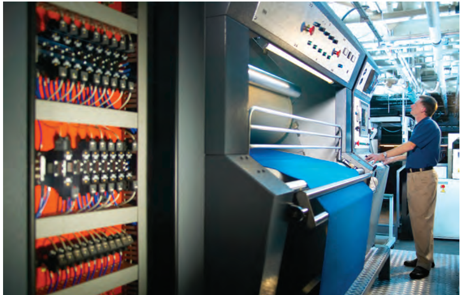
Batch Decatising. Additional finish is applied using this batch system. The levels of press are increased by this process and again made permanent by the high setting temperature.
